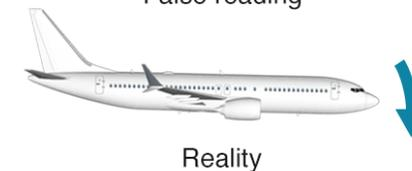
4. But if the sensor reading is wrong, MCAS may activate and push the nose down anyway
