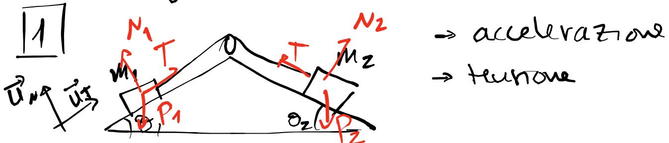
$$\text{for } p_1 \quad \left. \begin{array}{l} T - |P_1| \sin \theta_1 = M_1 a \\ \end{array} \right\}$$
