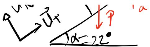
$$\begin{aligned} \vec{U}_T & \left\{ F + F_a - P_T = 0 \right. \\ \vec{U}_N & \left. N - P_N = 0 \right. \\ & \left\{ F + \mu_s N - Mg \sin \alpha = 0 \right. \\ & \quad \quad \quad \left. P_T \right. \\ N &= Mg \cos \alpha \\ & \quad \quad \quad \left. P_N \right. \end{aligned}$$
