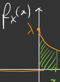
$$\begin{aligned} F_X(x) \stackrel{x>0}{=} \int_{-\infty}^x f_X(y) dy &= \int_0^x \lambda e^{-\lambda y} dy = \left[ -e^{-\lambda y} \right]_0^x = \\ &= -e^{-\lambda x} - (-e^0) = 1 - e^{-\lambda x}, \quad x \geq 0 \end{aligned}$$
